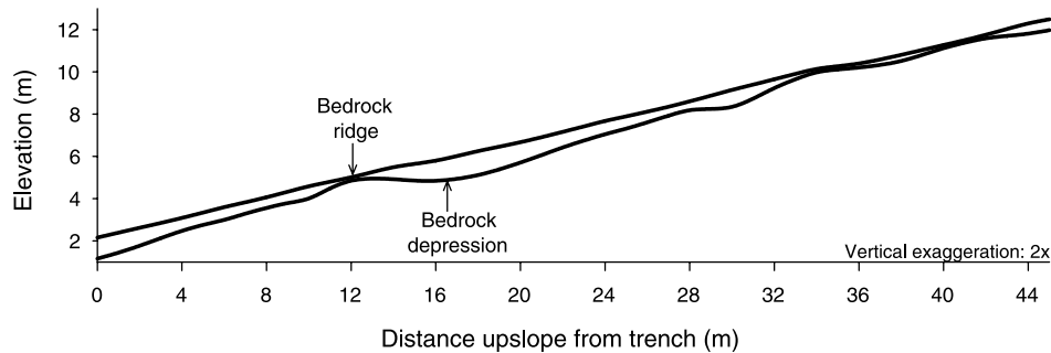
Figure 1. Surface and bedrock topography on a representative upslope transect across the hillslope.
